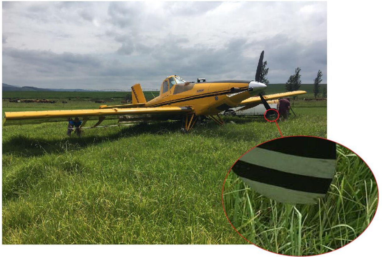
Figure 5: The damage sustained by the propeller.
