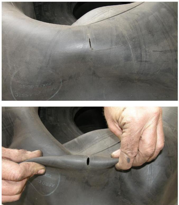
Figure 7: The deflated tube with the punctured area.
