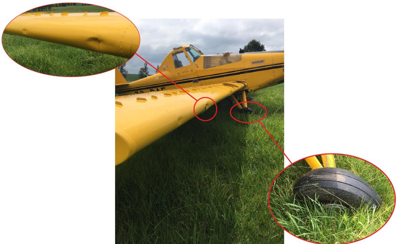
Figure 4: The deflated right tyre and damage caused to the right wing.
